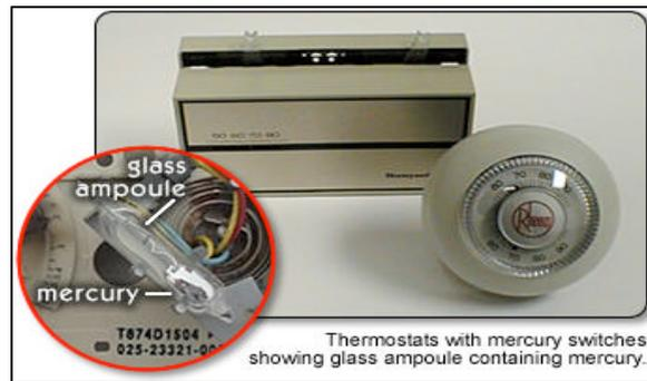
Mercury thermostats have bi-metal coils that contract and expand with room temperature. When the coil contracts or expands, it activates the mercury switch, which opens or closes a circuit to make the furnace, heat pump, or air conditioner turn on or off.<sup>7</sup>
